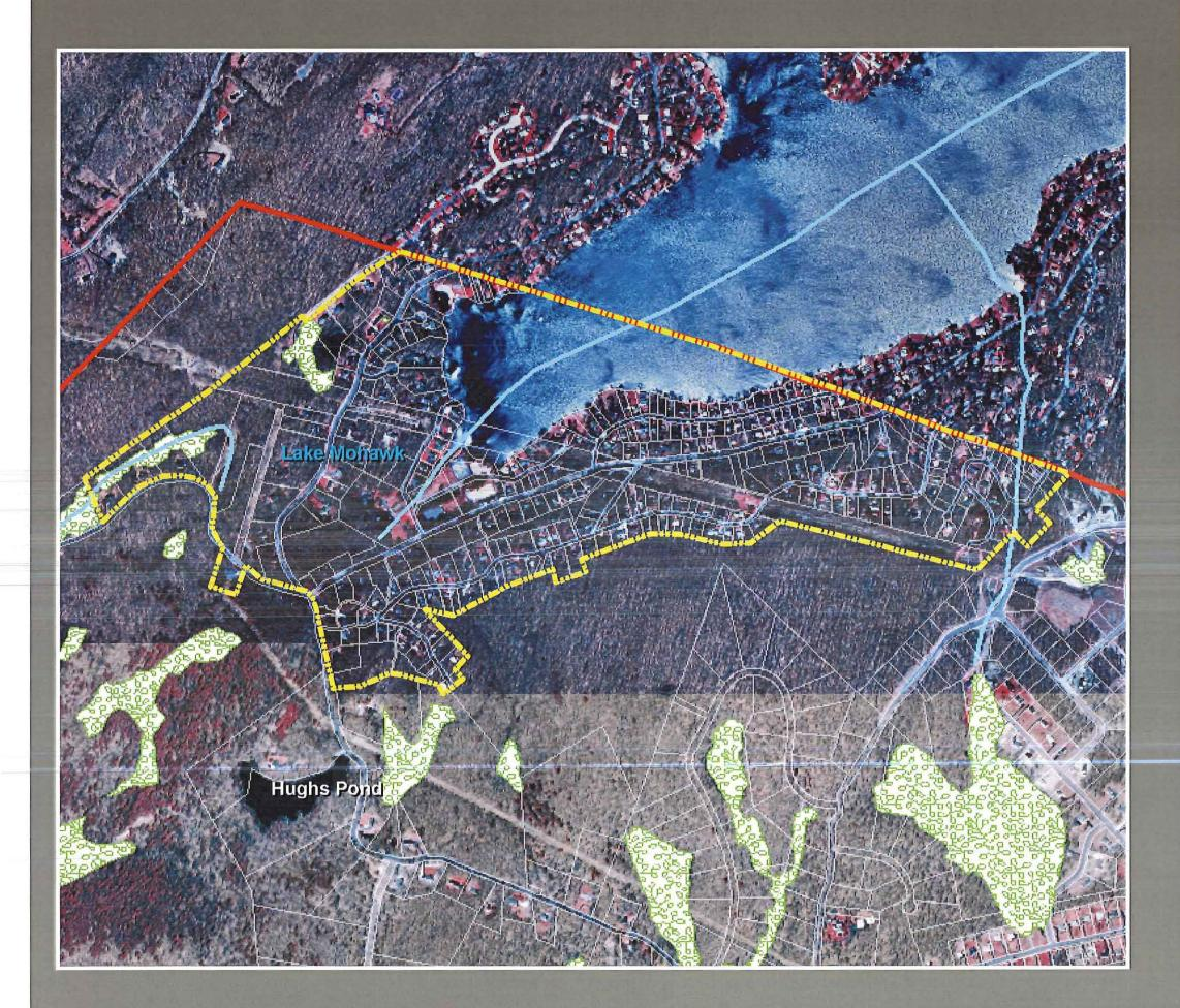
is close to the surface, are constrained from development and are unsuitable for various types of foundation construction and septic systems. Sufficient soil depth from the bottom of the septic system disposal bed to the top of the water table is necessary if septic inputs such as phosphorous, nitrogen and bacteria are to be prevented from leaching into the lake water.
